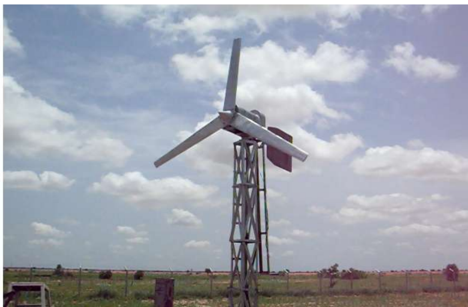
Figure 4 The HAWT Blade on a 4 meter Tower at the site.
